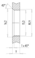
Installation direction: o-ring sits on chamfer.
